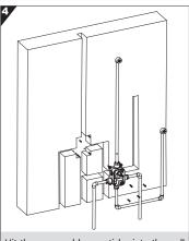
Hit the green rubber particles into the wall and lock the main body with screws Fix it tightly to the wall.
