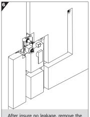
After insure no leakage, remove the handle wheel and handle.
