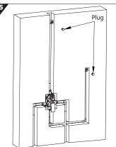
The handle and diverter wheel are prescrewed on the product, and then the plug need to be thread into the water outlet connector. Test the water normally to insure there is no water leakage.
